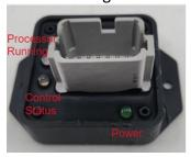
208-06-5566Y2 module that works on 1.5.0 and newer software (needs control type
