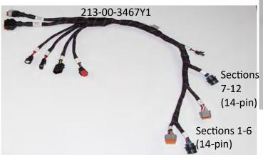
The 14-pin section connector on any SureFire JDRC 2000 Adapter Harness can plug into the LiquiShift 14-pin. Single Section LiquiShift eliminates the Manifold Controller found in multiple section LiquiShift systems. The A and B valves are controlled directly by the MultiTube Controller.
