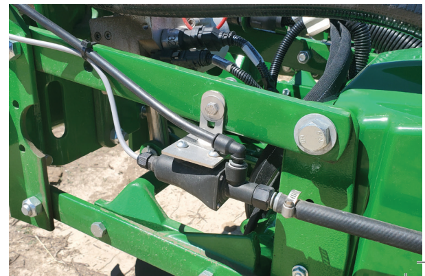
Row Control valve adjusts the flow to each individual row.
