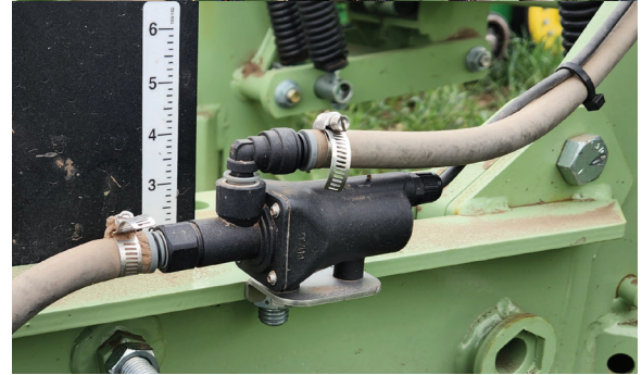
Row Control valve adjusts the flow to each individual row.
