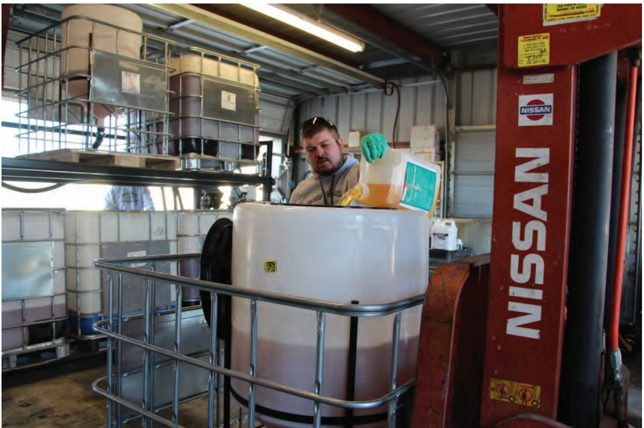
Cone tanks mounted in cage pallets for pouring-up jug product to be metered in bulk by QuickDraw.
