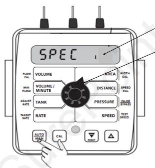
This number tells you which special CAL screen you are on. Pressing the CAL button will change this number. Quick Setup is on Page 1, with dial turned to AREA.
