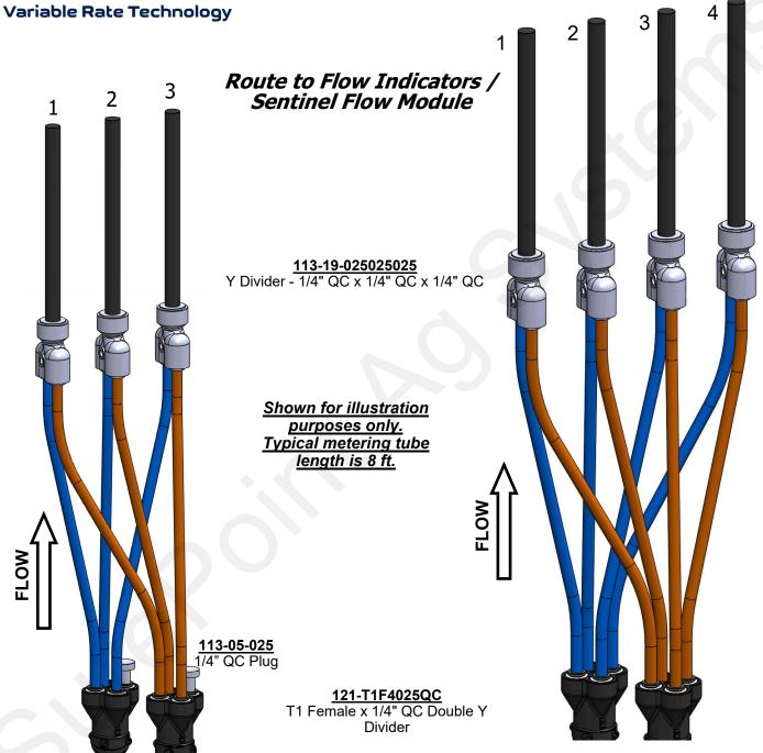
Double Y Dividers mounted to modular manifold
