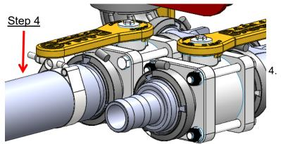
Route 2" hose from 105-200BRB to other tank. Use the 105-200150BRB for PumpRight or Tower. Use 105-200PLG075 and 101-075075 exclusively for use with Tower.
