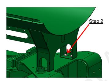
Loosely mount the back of 450-5000Y1 to the bolt plate on the hitch using four (4) 3/4" x 2-1/2" hex head bolts, washers, and flange nuts.
