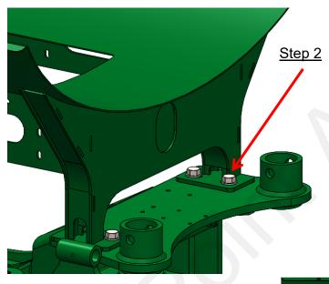
Loosely mount the back of 450-5093Y1 - 400 Gallon Tank Bracket to the bolt plate on the hitch using four (4) 3/4" x 2-1/2" hex head bolts, washers and flange nuts.
