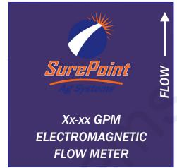
Flow Meters sold beginning October, 2012. Label is white lettering on blue background. 3-pin MP Shroud connector on pigtail.
