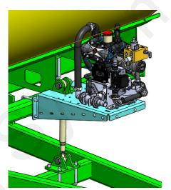
PumpRight pumps are fed with 1-1/2" hose from the valve in the plumbing kit below
