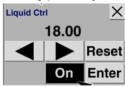
Press on the left arrow to decrease the applied rate by the Delta App Rate set during setup.
