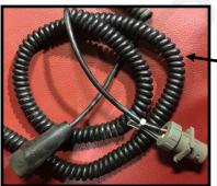
Tether switch from Case. Connects to connector on back of planter (Jump across these two pins on planter connector to activate pump without tether
