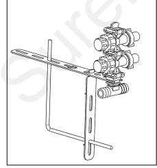
bracket on the rear of a bar. The check valve is mounted over the top of the bar. The supply line would run above and behind the bar. The short bracket is placed the notch to mount the check valve closer to the bar.
