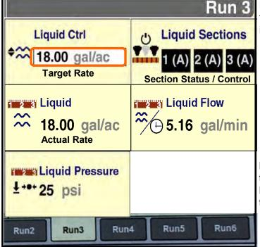
**Liquid Ctrl** (Liquid Control) - Use this to set the liquid fertilizer applied rate (Target Rate). Press on the box in the middle to bring up the following window:
