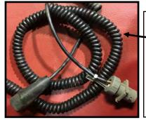
Tether switch from Case. Connects to connector on back of planter (Jump across these two pins on planter connector to activate pump without tether switch)
