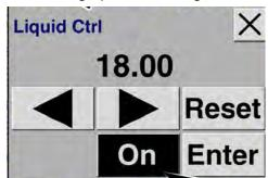
Press on the left arrow to decrease the applied rate by the Delta App Rate set during setup.
