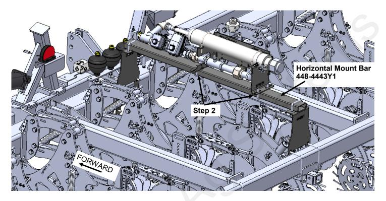
1. Repeat steps 1 and 2 from page 3. When mounting the Torpedo, parts that will NOT be used from kit 516-04-600100 are as follows...
