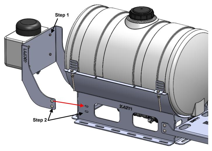
**Step 1:** Mount 3 Gallon Rinse Tank (727-05-SP0003-RT-Black) to 470-4307Y1 or 470-4308Y1 Rinse Tank Bracket. Use the supplied 5/16"x1/2" Bolts and Lock Washers to fasten.
