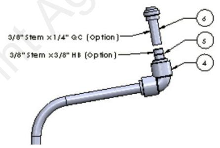
Included in the kit are quick connect plumbing fittings to attach the row plumbing to the fertilizer tube, whether it be for 1/4" metering tube, 3/8" tubing or 3/8" hose. See parts diagram above and/or page 1 for reference.
