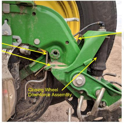
Inlet of Tube is shortened due to air bag support being in the way. Tip: Install tube with the 3/8" Quick Connect 90 deg elbow (113-10-038038) already installed before feeding up through row unit.
