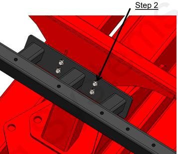
2. Loosely mount the 420-3797Y1 rear bulk fill support tank mount to the bolt plate on the rear CCS support using four (4) 1/2" x 1-1/2" hex head bolts, washers and flange nuts.
