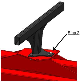
Loosely mount the 420-5433Y1 to the bolt plate on the rear bulk fill support using four (4) 3/4" x 3" hex head bolts, washers, and nylock nuts.
