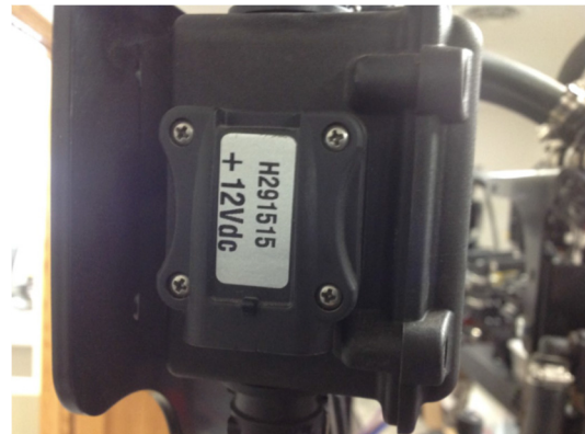
Figure 2: Plug in CAN DEVICE connector here.
