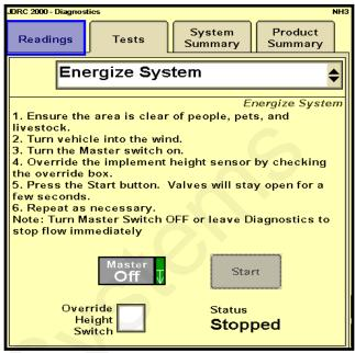
See the John Deere Rate Controller 2000 Operator's Manual for complete information on the setup and operation of the system.
