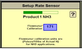
Flowmeter Calibration units are Pulses per 10 lbs of N. Your number may be different than above. pulses / 10 lbs = ((?) pulses / 10 gallons) / 4.22
