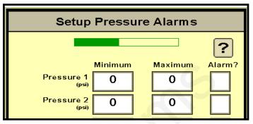
Set up as desired. If you put a check mark in the Alarm box, the system will not operate below that Minimum Pressure or above that Maximum Pressure. This may keep you above or below your Target Rate.
