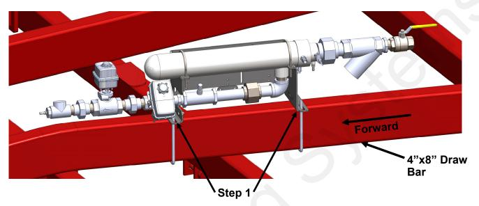
1. Mount the Torpedo to the 4"x8" Draw Bar using the provided 1/2"x4"x9-1/2" Square Bent U-bolts (380-1032). Tighten all nuts once Torpedo is in desired position along the 4'x8" Bar and clearance/interference of existing equipment has been checked.
