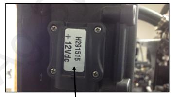
Plug in CAN DEVICE connector here
