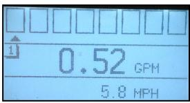
Arrow under Row 1 means the flow in Row 1 is 0.52 GPM.
