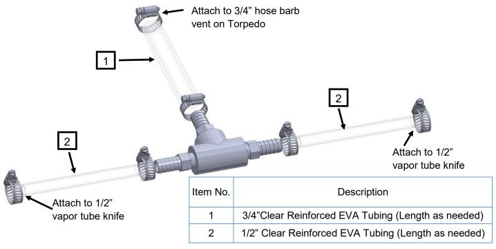
The Torpedo heat exchanger has (2) 3/4" dump outlet hose barbs near the inlet end to vent the vapor that is used to cool the heat exchanger. Each of these hose barbs can be connected to a 3/4" hose that will be connected to a vapor tube on a knife. Some applicators prefer to split each of these 3/4" vapor hoses to (2) 1/2" hoses so that the vapor is sent through four vapor tubes to the ground. Two of these kits are needed to convert from (2) 3/4" vapor tubes to (4) 1/2" vapor tubes.
