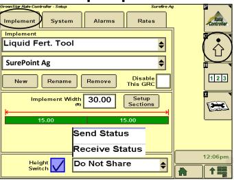
Set up Height Switch as appropriate for this system
