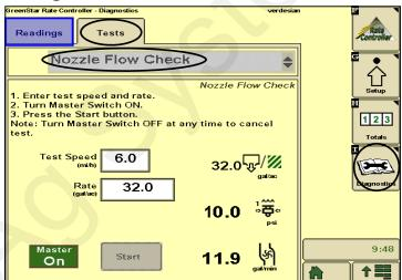
Use Nozzle Flow Check to see if system will lock on to a rate at a test speed. Pressure with water will be a lot lower than it will be with a heavier, thicker product.
