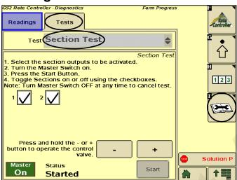
Section Test (or Calibrate PWM Limits) can be used for manual operation of the system. It can be used to prime the pump on startup, to rinse the system, or for troubleshooting.
