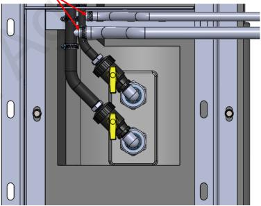
4. Using 1/2" and 3/4" hose barb tee fittings, connect hoses from second tank to first tank hoses as shown. Tighten all hose clamps.
