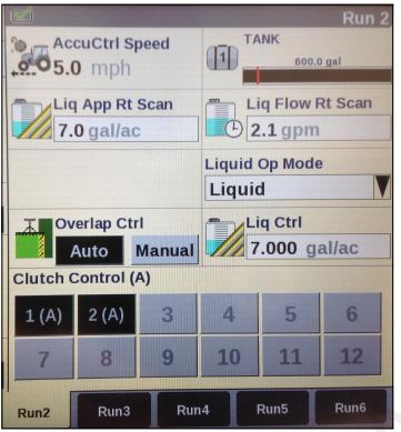
To use default AccuCtrl speed, turn Radar off. Toolbox > Vehicle > Radar Installed > NO
