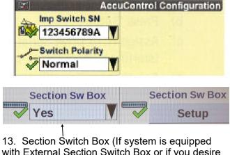
with External Section Switch Box or if you desire Manual Valve Section Control through Run Screens).
