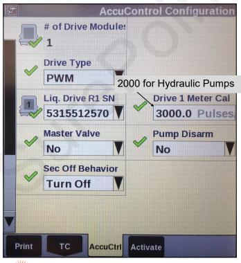
Start with these Valve Cal settings Work Condition > Valve Cal > Advanced Calibration
