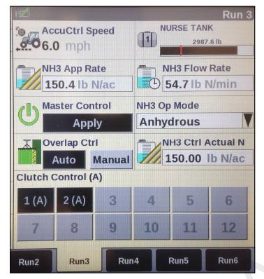
To use default AccuCtrl speed, turn Radar off.
