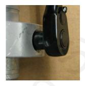
These orifices can be swapped out for different sizes depending on your application needs. Select the correct orifice based on your application needs by referring to the chart below.
