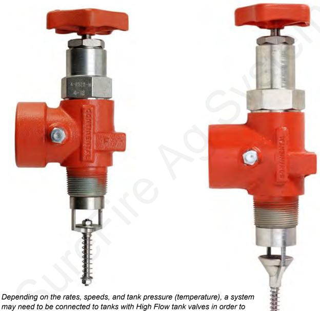
Depending on the rates, speeds, and tank pressure (temperature), a system may need to be connected to tanks with High Flow tank valves in order to allow enough product flow. The entire plumbing arrangement (valves, hoses, connections) must have high flow capacity in order to maximize flow to reach high rates at high speeds and cold temperatures.
