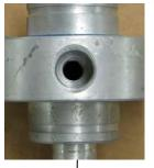
Threaded orifice not installed
