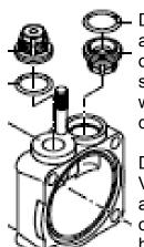
D70 - D115 Valves are on same side of head. Valves should pop out with slight screwdriver pressure.
