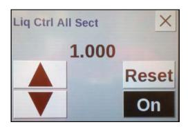
PWM Voltage—should increase as target rate is changed from 0 to 1. Voltage should end up around 13 volts.
