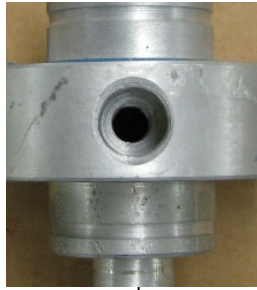
Threaded orifice not installed
