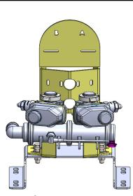
Valve Stack can mount directly to forward/ backward frame. Use optional bracket kit 515-105100 to mount valve stack to lateral frame members. Feed into the section valve stack using 3/4", 1", or 1-1/2" hose from the pump. Each section valve output hose may be split using tees or crosses to feed the necessary number of banks per section.
