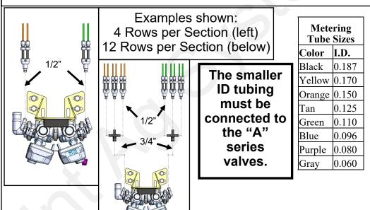
Dual metering tube comes pre-assembled in 3, 4, or 6 row assemblies. 1/2" hose barb ends go to the section valves, 3/8" tubing goes to flow indicators.
