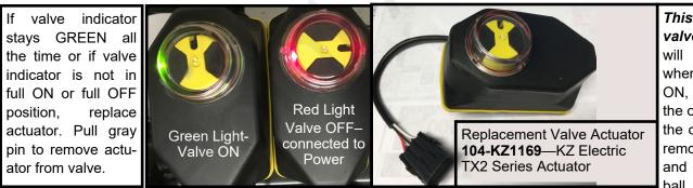
*This is a 3-way valve*. If product will not flow when valve is ON, either move the outlet hose to the other port, or remove actuator and rotate valve ball 180°, and replace actuator.
