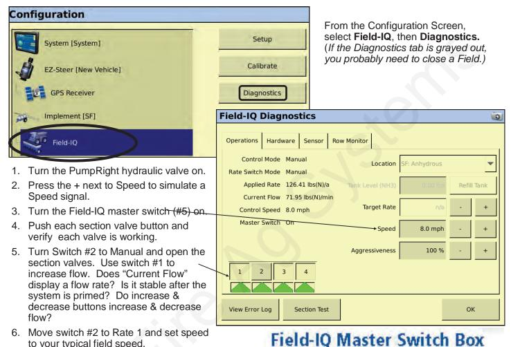
6. Move switch #2 to Rate 1 and set speed to your typical field speed.
