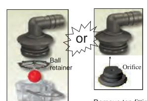
If using a metering orifice in the flow indicator, the orifice replaces the ball retainer. If not using an orifice here, the ball retainer must be in place.
