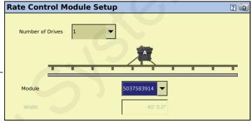
Set the Valve Setup as shown.
