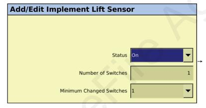
If using an Implement Lift Switch, change the Status to **On**. Enter the number of switches and the minimum number of switches that need to change. You will need to Calibrate the Implement Lift Switch later on by going to Field IQ - Configuration - Implement Lift Switch (see page 28 and page 59.)
