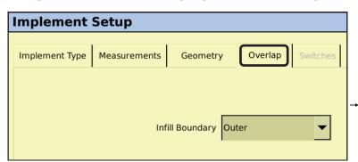
Select either "Outer" or "Inner" for the Infill Boundary on the Overlap Tab.
