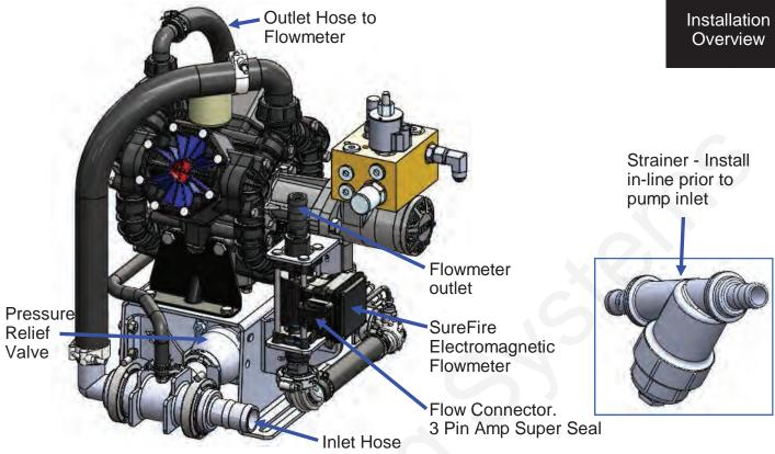
**Inlet:** The PR17 and PR30 PumpRight are shipped with a 1 1/2" inlet hose barb. Attach this to the hose from your supply tank and strainer. A 1 1/2" 90 degree hose barb is included and can be substituted. **Inlet Strainer:** A 20 mesh strainer is included in the pump kit. The manifold strainer includes two hose barbs so it can be mounted anywhere in the inlet line. If space allows, the strainer can be mounted directly to the inlet plumbing assembly as shown below.
