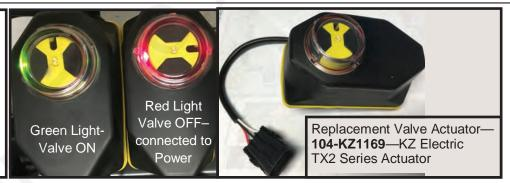
**This is a 3-way valve.** If product will not flow when valve is ON, either move the outlet hose to the other outlet port, or remove actuator and rotate valve ball 180°, and replace actuator. Product should flow through the port closest to the Indicator light when the valve is open (green).
