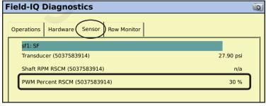
The **Sensor** tab provides information on the Pressure Sensor and Pump Speed (PWM Percent). It is good to know the **PWM Percent** required for normal operation.
