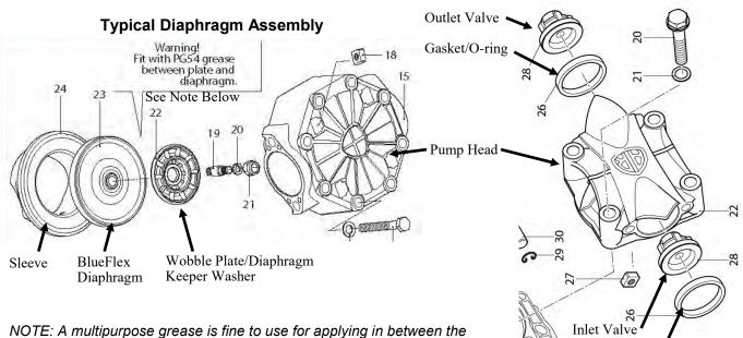
NOTE: A multipurpose grease is fine to use for applying in betwe Diaphragm and Wobble Plate/Washer
