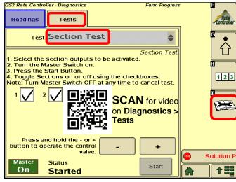
Section Test or Calibrate PWM Limits can be used for manual operation of the system. Calibrate PWM Limits is good to prime the pump on startup, to rinse the system, and for troubleshooting.
