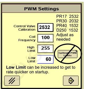
The "Calibrate PWM Limits" button is not necessary after you enter the numbers above. However, the Calibrate PWM Limits Test can be used to test the system in a manual mode.
