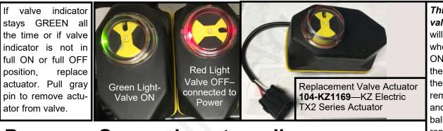
*This is a 3-way valve*. If product will not flow when valve is ON, either move the outlet hose to the other port, or remove actuator and rotate valve ball 180°, and replace actuator.
