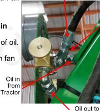
Hydraulic Tee fitting 161-03-8MJ-8MJ-8FJXT Oil return to Tractor
