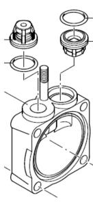
D70 - D115 Valves are on same side of head. Valves should pop out with slight screwdriver pressure.
