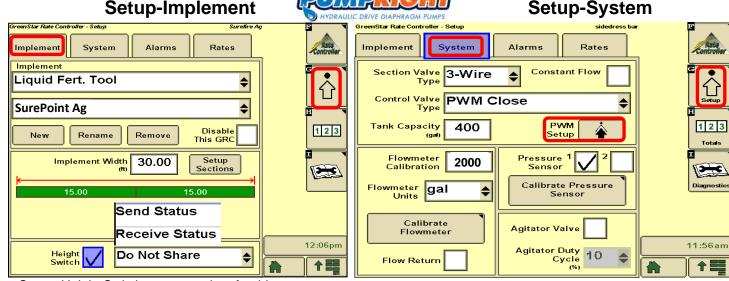
Set up Height Switch as appropriate for this system. Some systems may not use a height switch.
