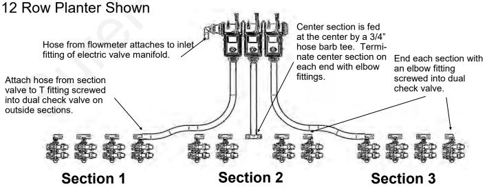
For a **<u>2 section plumbing system</u>**, omit the center section and plumb similar to the outside 2 sections.
