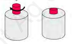
Preseason - Clean the dirt out of the stem for the red knob so the red knob can be moved by hand. Be sure to lock it in the down position before operating the pump.
