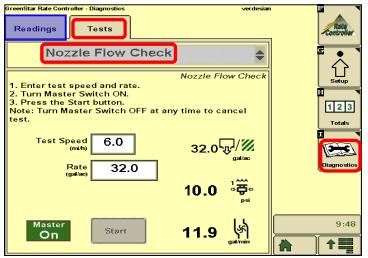
Use **Nozzle Flow Check** to see if system will lock on to a rate at a test speed. Pressure with water will be a lot lower than it will be with a heavier product. Some check valves may not open with low pressure.
