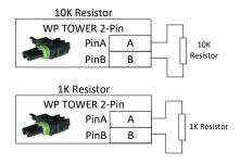
This harness can be set to pull the signal wire up to 12V or down to GND through the included resistors. The meter type must be determined before the user can wire up and use this harness. Consult Instruction Sheet 396-3723Y1 for configurations.
