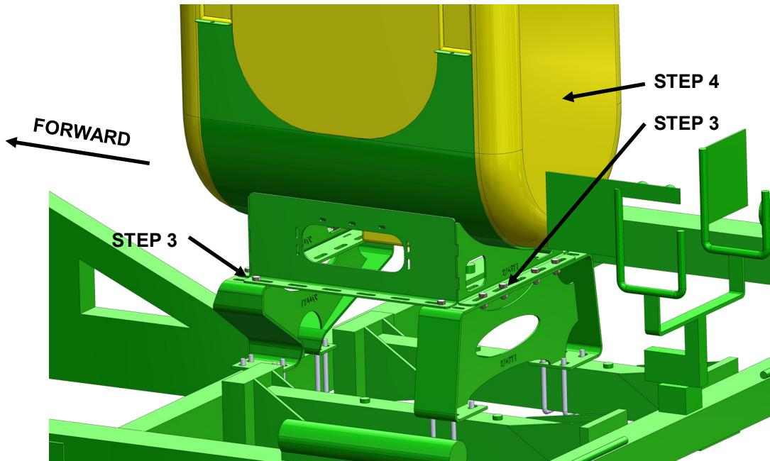
3. Mount the Tank Cradle (421-2763Y1) to the Tank Stands as shown in picture above with the provided 5/8" Bolts (300-100108-5) and Flange Nuts (323-10). Fully tighten all Nuts and U-bolts.
