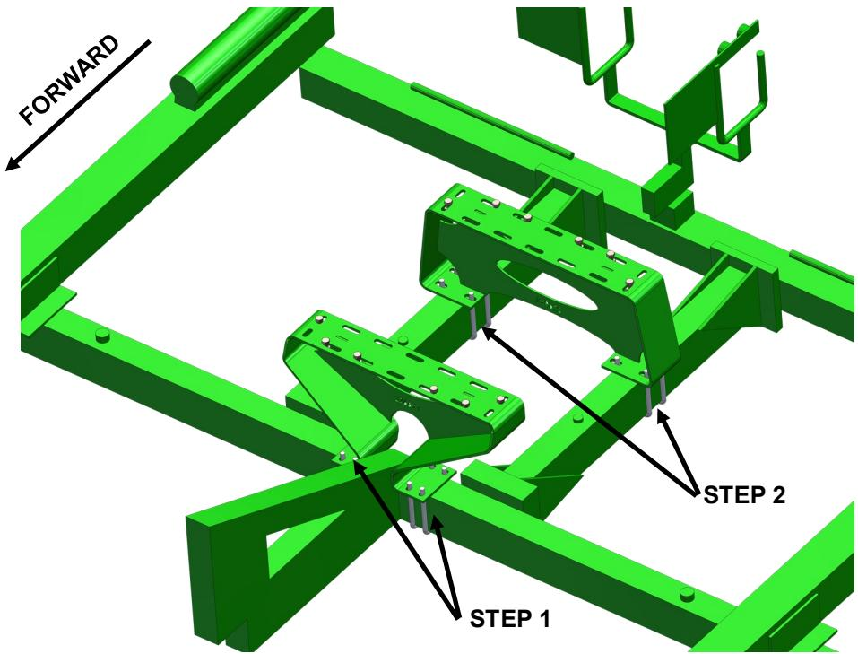
1. Mount the Front Tank Stand (420-2766Y1) with the supplied Square Bend U-bolts (380-1041) as shown in picture above. Fully tighten U-bolts.
