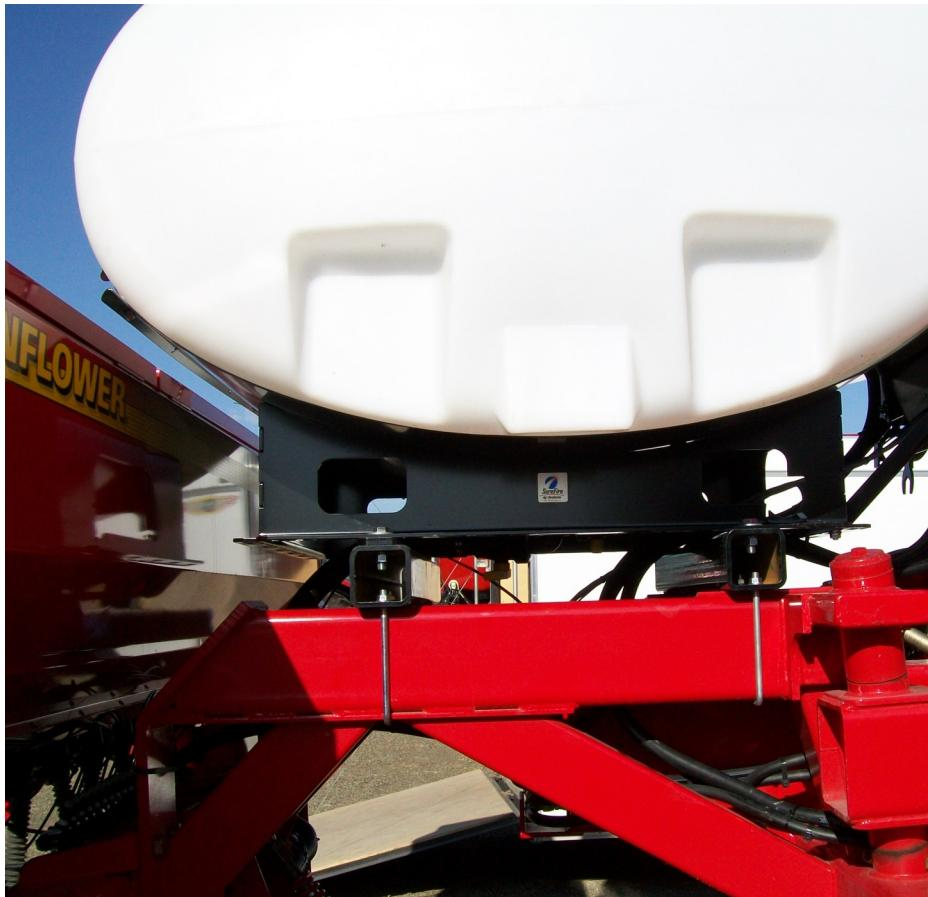
3. Set the tank cradle on the 4"x4" supports. Bolt down with 5/8" bolts (2" bolts in the front, 2-1/2" bolts in the rear), washers, and flange nuts.
