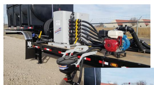
QuickDraw on dropdeck. Front and rear water storage. Electric 3" hose reel and locations for 6 chemical totes.
