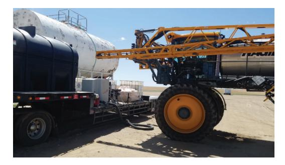
QuickDraw installed on sprayer transport trailer.
