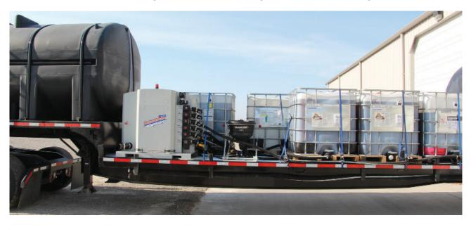
QuickDraw on drop-deck trailer. Water tanks front and back. Locations for 7 chemical totes. QD swing-down eductor for ground level working.
