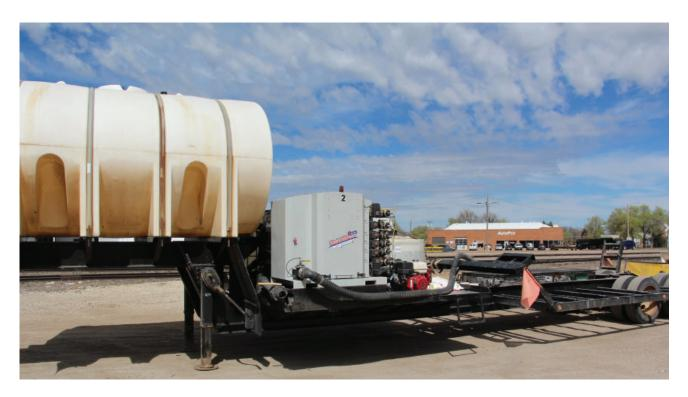
QuickDraw installed on sprayer transport trailer.
